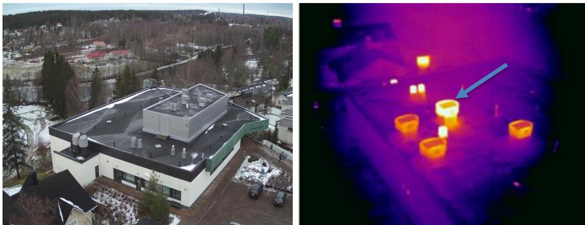
**Figure 1: Aerial view of the Karhula swimming hall on the left [6] and a thermal image of the exhaust air diffuser on the roof of the swimming hall on the right, where the examined unit is marked with a blue arrow [7]**
