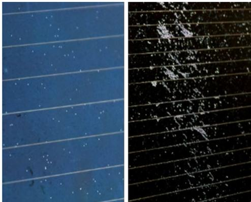
**Figure 16:** Left: Small white spots in M04 (front contact) after 165 hours of Bias Damp Heat Testing at  $-1000$  V. Right: TCO delamination in M04 (front contact) after 410 hours of Bias Damp Heat Testing at  $-1000$  V.
