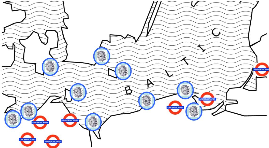
The Pelton turbine symbolizes spots for PHS at steep coast stages. The Underground label symbolizes potential underground layers which are suitable for caverns. This map is not thought to give exact places for the proposed storage solution but to show the potential in the South Baltic Region. Higher interests like environmental protection, spatial planning and elector's decisions have to be respected in forehand.
