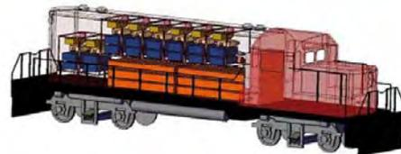
Conceptual design of fuelcell road-switcher employing 12 MW PEM fuelcells (blue) and storage of 250 kg of hydrogen in a revised steel metal hydride (orange)
