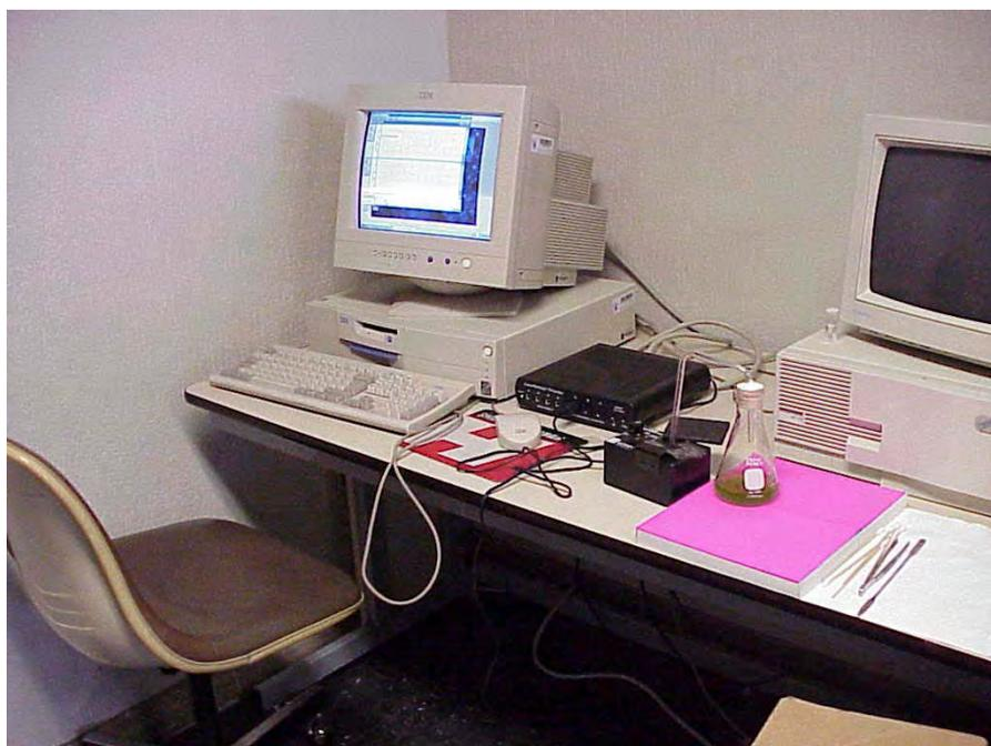
*Fig.3 Hydrogen detection system showing alga recipient, glass tube, colorimeter, interface and PC.*
