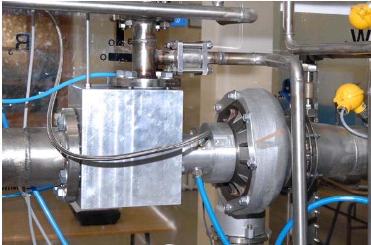
Fig. 2 General view of the high speed turbine and centrifugal compressor set
