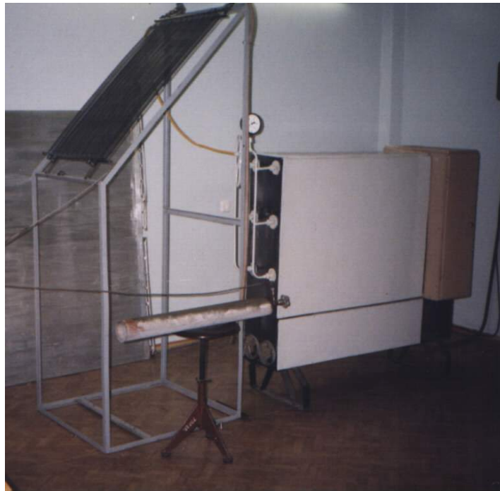
Fig. 13. Six adsorbers sorption cooler (3+3) with the evaporator/condenser for heating/cooling in tri-generation system.
